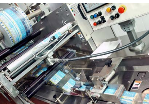
One of Galaxy's individually wrapped slice (IWS) machines
